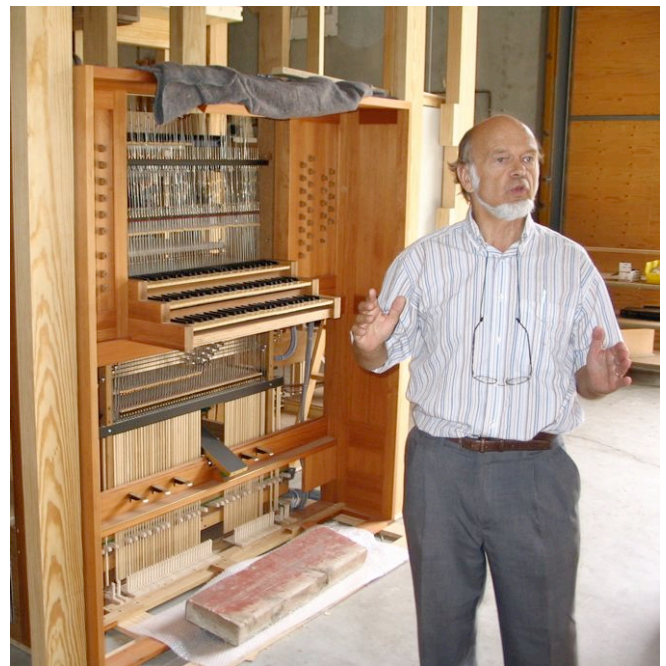
Gerhard Grenzing, Barcelona, with organ showing typical tracker action leading from the keys to the valves which cause the organ to play.
